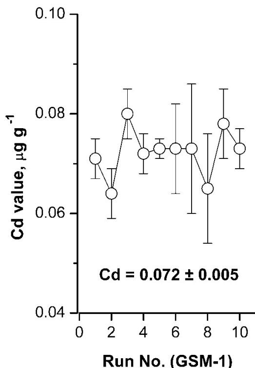
**Fig.S2.** Stability of Cd values obtained by aerosol dilution ICP-MS in SRM GSM-1. Mean  $\pm$  SD, the SD is the standard deviation for ten separate aliquots of the samples analyzed over a period of three months. The error bars in Figure were defined as the standard deviation for 3 replicates in single analysis.
