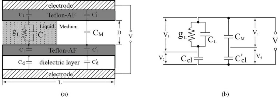
**Fig. S1** (a) Equivalent circuit model for parallel-plate microfluidic device. (b) Simplified circuit for the model. Tefflon-AF layer on top plate and Tefflon-AF/SOG layers on bottom plate are grouped together and represented by one capacitor.
