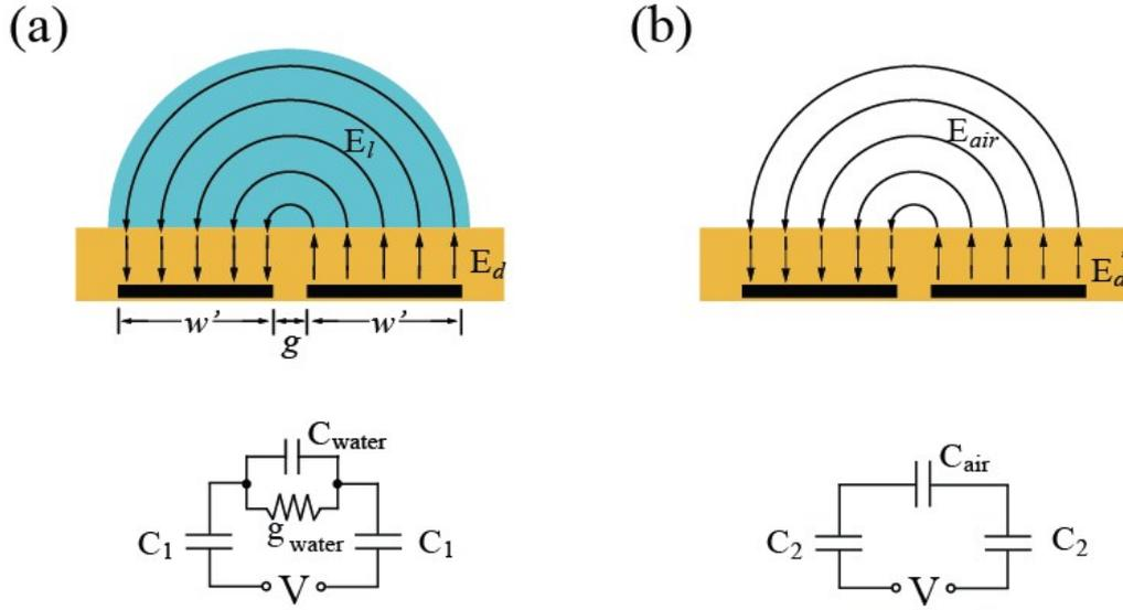
**Fig. S2** Approximate E-field distribution on coplanar electrode structure and corresponding circuit model. (a) The liquid filled region. (b) The air filled region.
