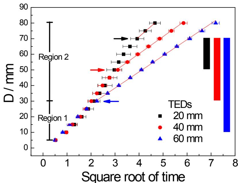
**Figure S3.** Distance traveled by the fluid over the square root of time using TEDs of different lengths. The paper-based strips were positioned vertically.
