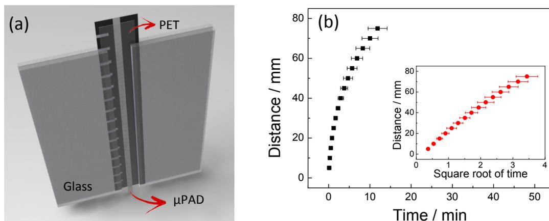
**Figure S2.** Distance traveled by the fluid inside the paper channel over the time for the  $\mu$ PADs sealed without charges. *Inside:* the distance traveled by the fluid over the square root of time.
