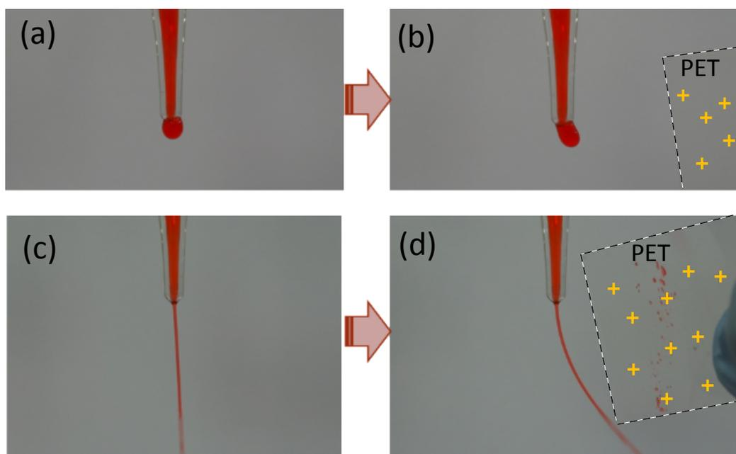
**Figure S1.** (a) Pendant drop of a food-dye solution inside a glass burette and (b) its deforming by approximation of tribocharged PET sheets. Straight flow (c) and its shift (d) before and after the approximation of a charged PET sheet, respectively.
