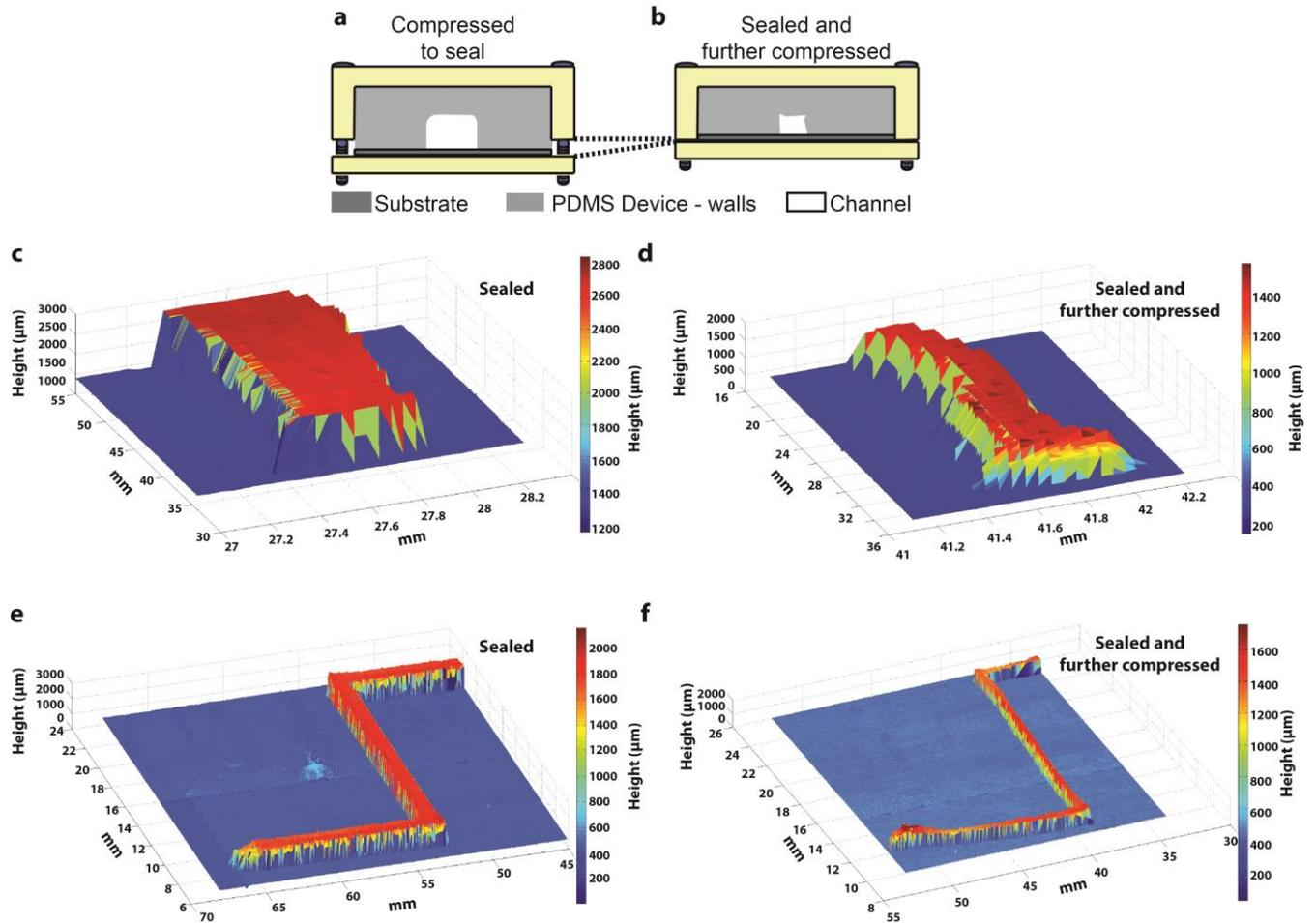
**Figure S5.** Data for the height and width measurements of the channels along XZ and YZ axes (a) plotted in Fig. 3. Tabulated data was obtained through profilometry of bismuth alloy replicates cast at varying pressures. Z is the height, XZ-width is the width of the channel perpendicular to X-axis and YZ-width is the width of the channel perpendicular to Y-axis. The devices used were fabricated in PDMS.
