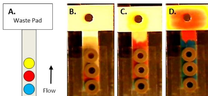
**Figure S7. Sequential delivery of buffers to enable a single end-user step.** A) Schematic. B-D) The images are taken from a video where three buffers were sequentially delivered to nitrocellulose. Yellow: capture buffer; red: wash buffer; blue: elution buffer. Using this method, our DNA concentration and purification system can be directly integrated with a simple user interface which requires only one step for activation<sup>62,63</sup>.
