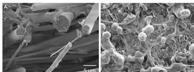
**Figure S1. SEM images of glass fiber and nitrocellulose used to determine membrane surface area for polymer adsorption studies.** SEM imaging and sputter coating work was performed at the University of Washington Nanotech User Facility (NTUF), a member of the NSF-sponsored National Nanotechnology Infrastructure Network (NNIN). A) Glass fiber. B) Nitrocellulose.
