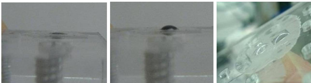
**Fig.S2:** Pressure induced inflation of the blister without a rigid backing
