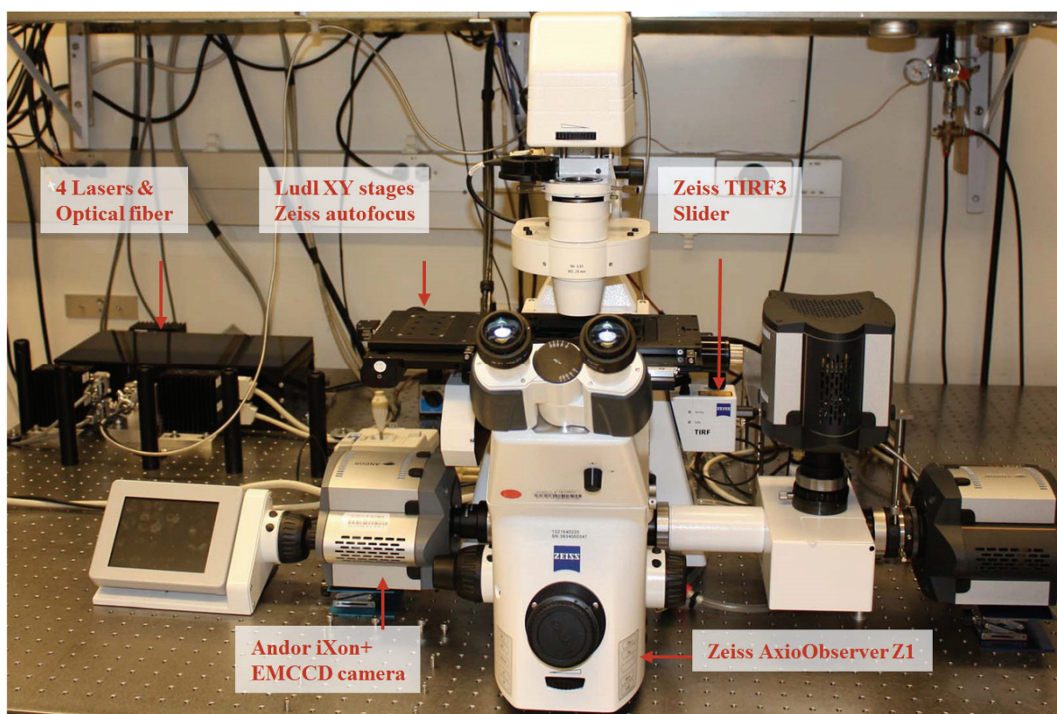
Fig.S1 Microscope system with a TIRF setup for single-molecule imaging and kinetics measurements. The system is based on a fully motorized inverted fluorescence microscope (Zeiss AxioObserver Z1). An adaptor (Zeiss RITF3 Slider) is used to introduce the laser excitation into the objective (100x oil, NA 1.46, Alpha Plan Apochromat, Zeiss). The lasers (405 nm direct diode, 488 nm direct diode, 532 nm DPSS and 642 nm direct diode lasers) are combined and coupled into the TIRF slider by a polarization preserving single-mode broadband optical fiber (kine-FLEX, Point Source).
