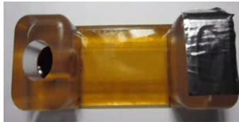
Step Two - Vacuum applied to waste chamber, sample begins movement through device
