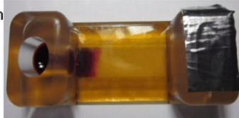
Step Three - Device runs until collection tub is filled with sedimented cells
