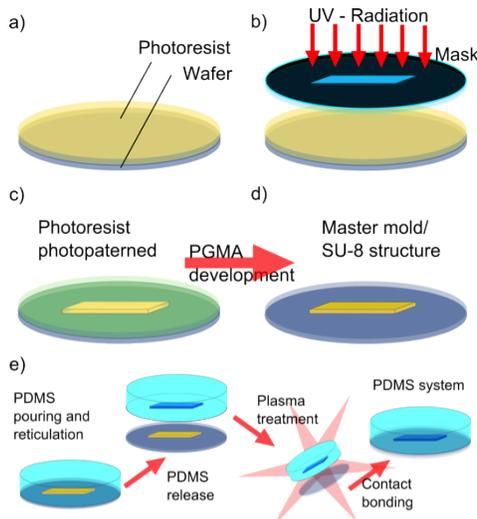
Fig. S1. (a) - (e) Schematic representation of the fabrication of a SU-8 mold and the casting and fabrication of a PDMS based microfluidic system.
