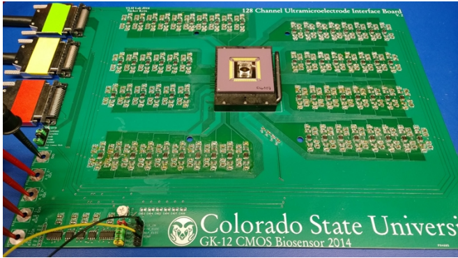
Supplementary Figure 7. Circuit board with the electrode array chip in the middle and other supporting circuits around it.
