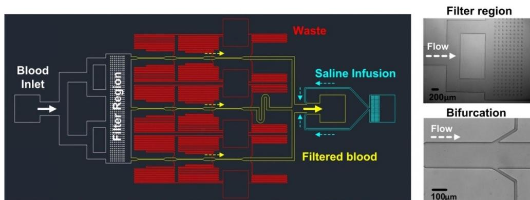
**Supplementary Figure S1** (*left*) CAD layout of the developed  $\mu$ BM device. Filtered blood flows along the main channels (yellow) towards a single outlet while marginated cell components are removed via the side channels (red) as waste. A saline infusion port (blue) is added next to the filtered outlet to compensate for volume loss. (*right*) Optical images of the inlet filter region and bifurcation at each stage.
