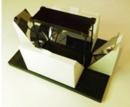
**Figure S2.** Manufacturing setup. (a) A 3D-sketch of the setup showing the roof, base, and the four angled blocks where mirrors are attached. (b) Photograph of the setup.
