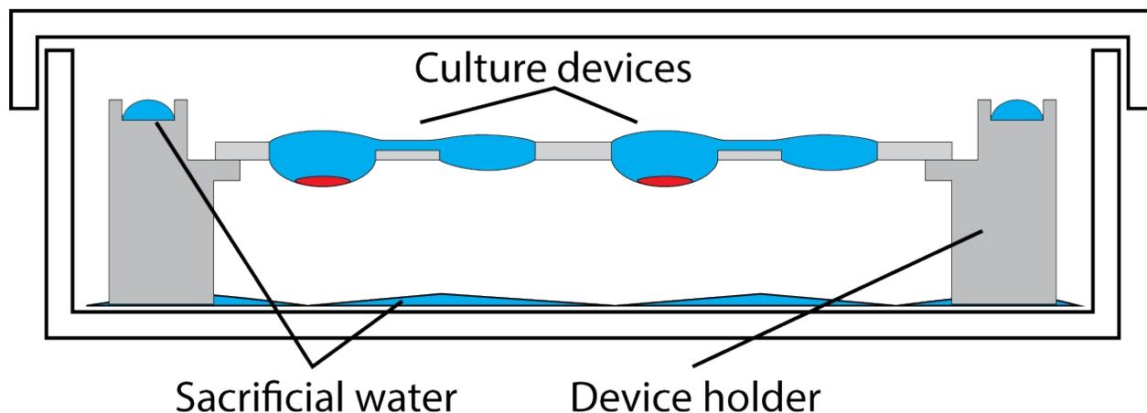
Figure S1. The device holder is placed in an OmniTray (Nunc) water is added to the bottom of the OmniTray and to the channel features of the device holder. The device is then placed into the device holder and filled with media and cells. The lid is placed on the OmniTray to ensure proper humidification of the device to prevent evaporation.
