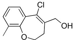
Colourless liquid, Yield 82%; R<sub>f</sub> 0.5 (Pet ether : EtOAc 1:9); MS m/z 225.1 (M+1, 100%); IR: 3465, 3025, 2886, 1627, 1491, 1411, 1295, 1046, 1029, 837; <sup>1</sup>H NMR (CDCl<sub>3</sub>, 400 MHz): δ 7.45 (d, 1H, J = 7.8 Hz), 7.20 (d, 1H, J = 7.9 Hz), 7.16 (t, 1H, J = 7.6 Hz), 4.58 (s, 2H), 4.54 (t, 2H, J
