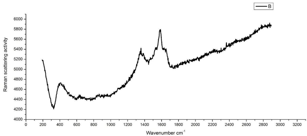
**Figure S5.** Raman spectrum of **5g** [Cu(L<sub>7</sub>)<sub>2</sub>Cl<sub>2</sub>]
