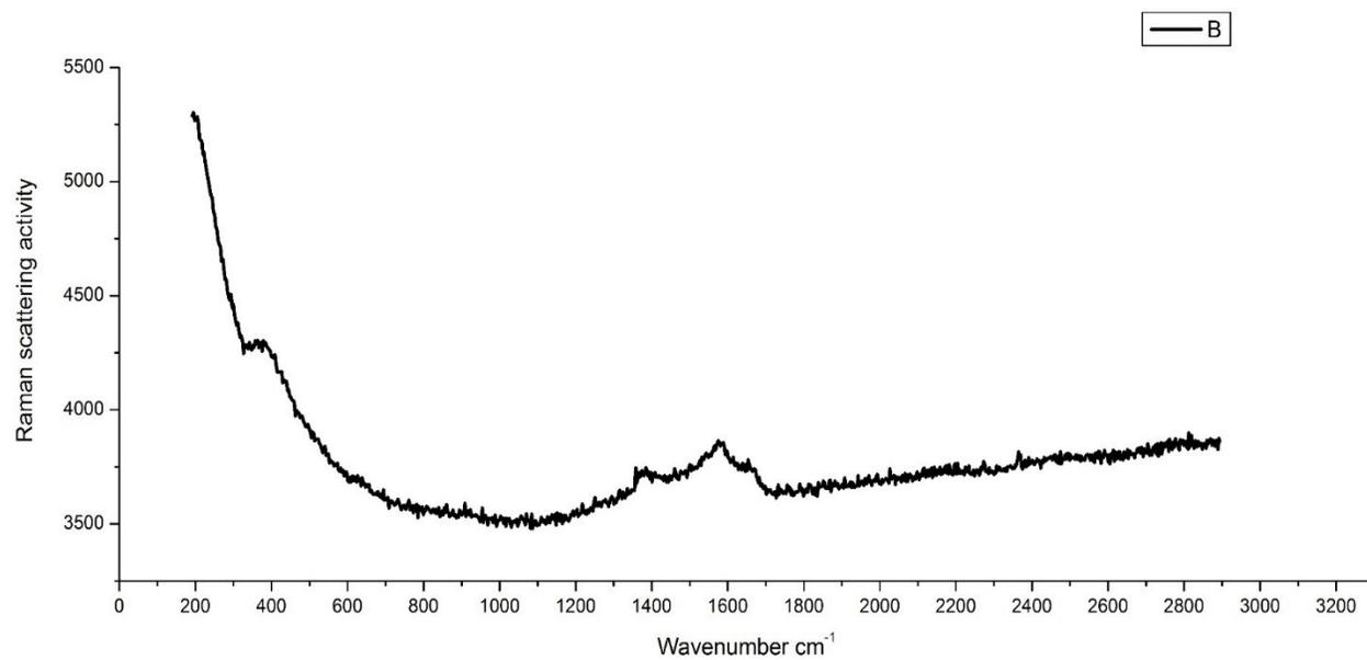
**Figure S2.** Raman spectrum of **5c** [Cu(L<sub>3</sub>)<sub>2</sub>Cl<sub>2</sub>]
