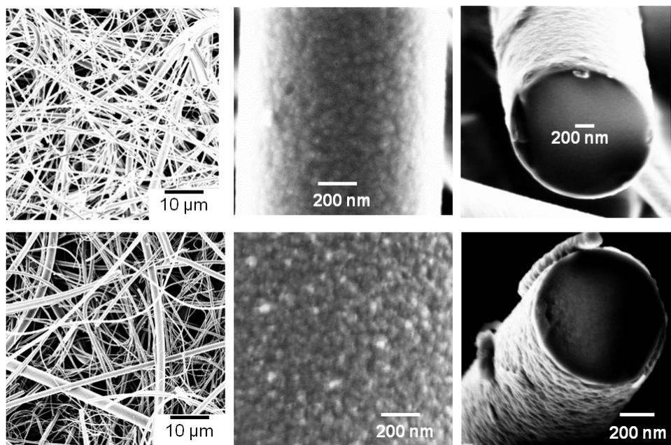
**Figure S1.** Scanning electron micrographs of the exterior surface (left), high resolution of a fiber surface (middle), and a cross section (right) of EP1 poly(V3D3)-C@SiO<sub>2</sub> FP (top row) and EP2 poly(V3D3)-C@SiO<sub>2</sub> FP (bottom row). Contrast and brightness settings are identical for all micrographs.
