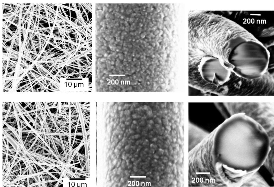
**Figure S2.** Scanning electron micrographs of the exterior surface (left), high resolution of a fiber surface (middle), and a cross section (right) of *iCVD1* poly(V3D3)-C@SiO<sub>2</sub> FP (top row) and *iCVD2* poly(V3D3)-C@SiO<sub>2</sub> FP (bottom row). Contrast and brightness settings are identical for all micrographs.
