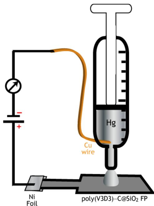
**Figure S3.** Schematic of the solid-state measurement setup with a liquid Hg probe.
