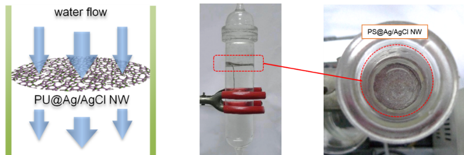
Figure S4. Apparatus for the water wash test of PS@Ag/AgCl NW with non-welded and welded Ag/AgCl NW network.
