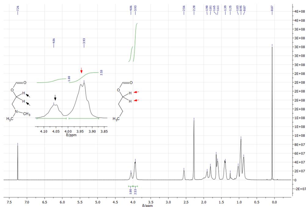
**Fig S8** The full  $^1\text{H}$  NMR spectrum of Poly(*n*-butyl methacrylate)-*block*-poly(2-(dimethylamino) ethyl methacrylate).
