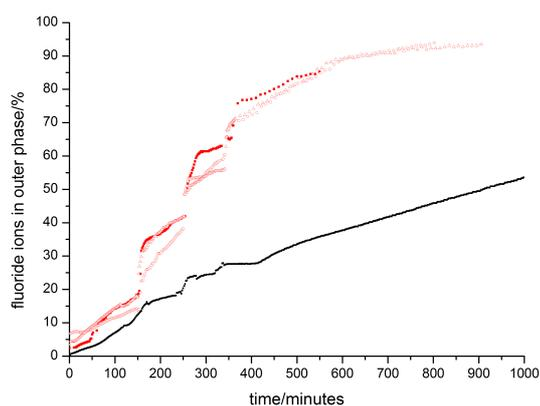
**Fig S7** Fluoride ion release of particle-embedded vesicles with hydrogen peroxide (red) and water (black) triggers at 150, 250 and 340 minutes.
