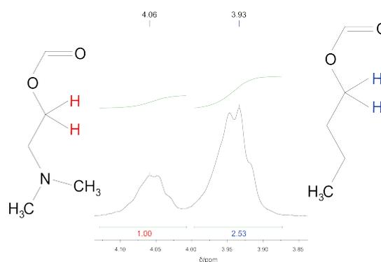
**Fig S2** The two proton environments used to assess block ratio alongside their  $^1\text{H}$  NMR peaks (See full spectra in appendix).
