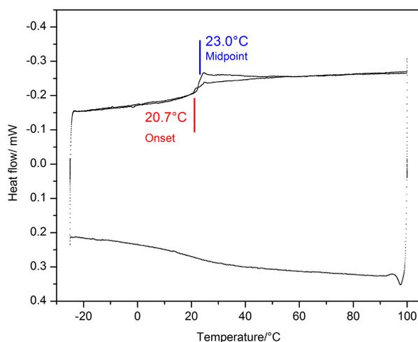
**Fig S3** The DSC curve of pBMA-b-pDMAEMA showing the onset and midpoint glass transition temperature.
