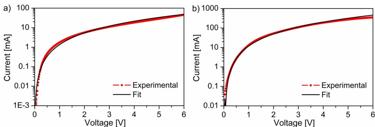
**Figure S2.** Experimental and fitted  $J$ - $V$  curves of the hole-only devices for (a) HTM **1** and (b) spiro-MeOTAD hole transporting materials.
