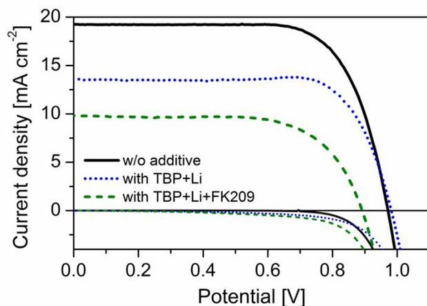
**Figure S3.**  $J$ - $V$  curves of devices using HTM **1** with additives and dopant. The best device without additives and dopant is included for comparison.
