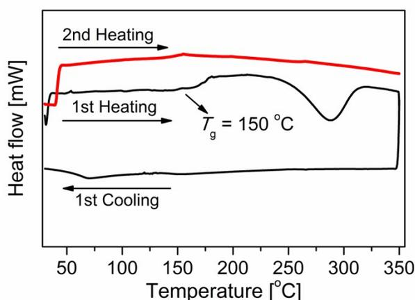
**Figure S1.** Differential scanning calorimetry (DSC) trace of HTM **1** measured under Ar flow at heating and cooling rate of 10 °C/min.
