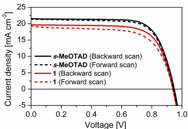
**Figure S5.** Current-voltage hysteresis curves of perovskite solar cells comprising champion devices with HTMs spiro-MeOTAD and spiro-CPDT **1** measured starting with backward scan and continuing with forward scan. The  $J$ - $V$  characteristics were measured with  $50 \text{ mV s}^{-1}$  scan rate at 1 sun illumination.
