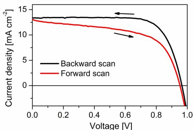
**Figure S4.** Current voltage hysteresis curves of perovskite solar cell device based HTM **1** containing *t*BP+Li as additives.
