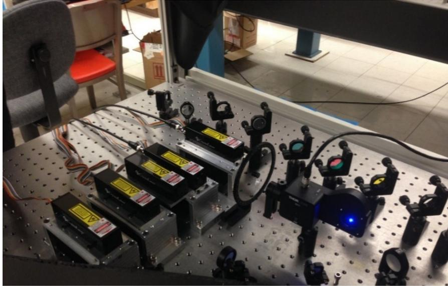
**Figure S6.** Laser guns (375, 473, 532, and 561 nm lasers all from *CrystaLaser*) for writing the information onto the photoswitchable thin films.
