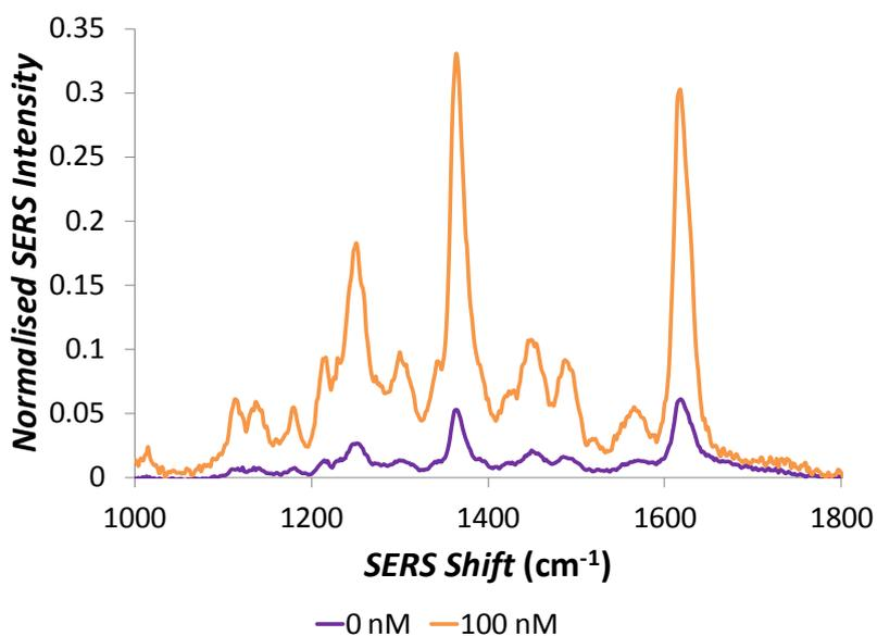
**Figure S6.** SERS spectra of RB1 coated gluconanoparticles 5 minutes before and after incubation with ConA in HB2. 514.5 nm excitation wavelength used, 1 second acquisition with 3 accumulations. The laser excitation wavelength used is 514.5 nm with a 1 second acquisition, 3 accumulations and 3 replicates measured.
