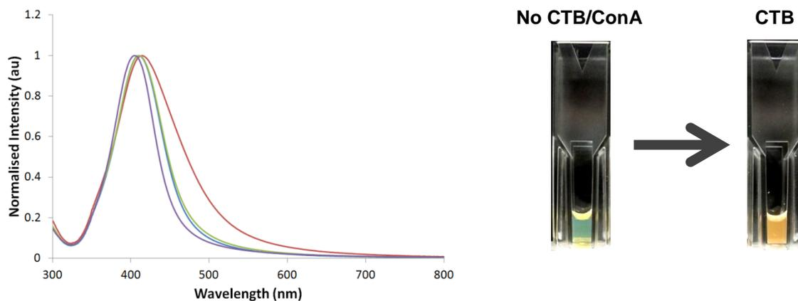
**Figure S4.** Extinction spectra of EDTA reduced colloid (purple), GSNPs (blue), GSNPs incubated with 80 nM ConA (green) and GSNPs incubated with 80 nM CTB (red). Photographs show cuvette containing GSNPs before and after addition of CTB (80 nM) in HB2.
