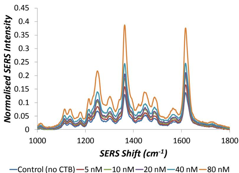
**Figure S5.** SERS spectra of RB1 coated GSNPs 5 minutes after incubation with CTB (in synthetic freshwater) at increasing concentrations (0-80 nM). 514.5 nm excitation wavelength used, 1 second acquisition with 3 accumulations. The laser excitation wavelength used is 514.5 nm with a 1 second acquisition, 3 accumulations and 5 replicates measured.
