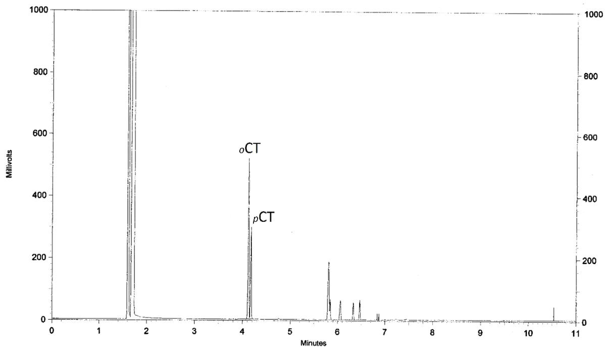
The GLC chromatogram of the reaction mixture of the chlorination of toluene using  $\text{KHSO}_5$  and  $\text{KCl}$  in the  $\text{CH}_3\text{OH}-\text{H}_2\text{O}$  solvent mixture.
