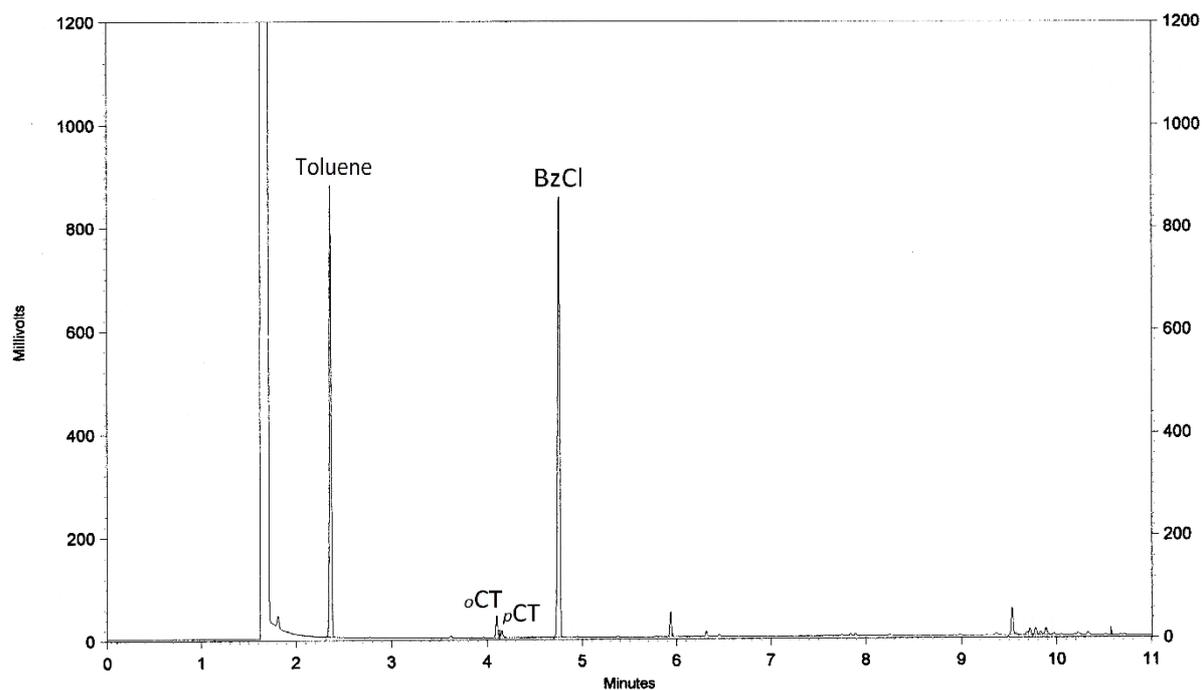
The GLC chromatogram of the reaction mixture of the chlorination of toluene using  $\text{KHSO}_5$  and  $\text{KCl}$  in the  $\text{CH}_2\text{Cl}_2$ - $\text{H}_2\text{O}$  solvent mixture.
