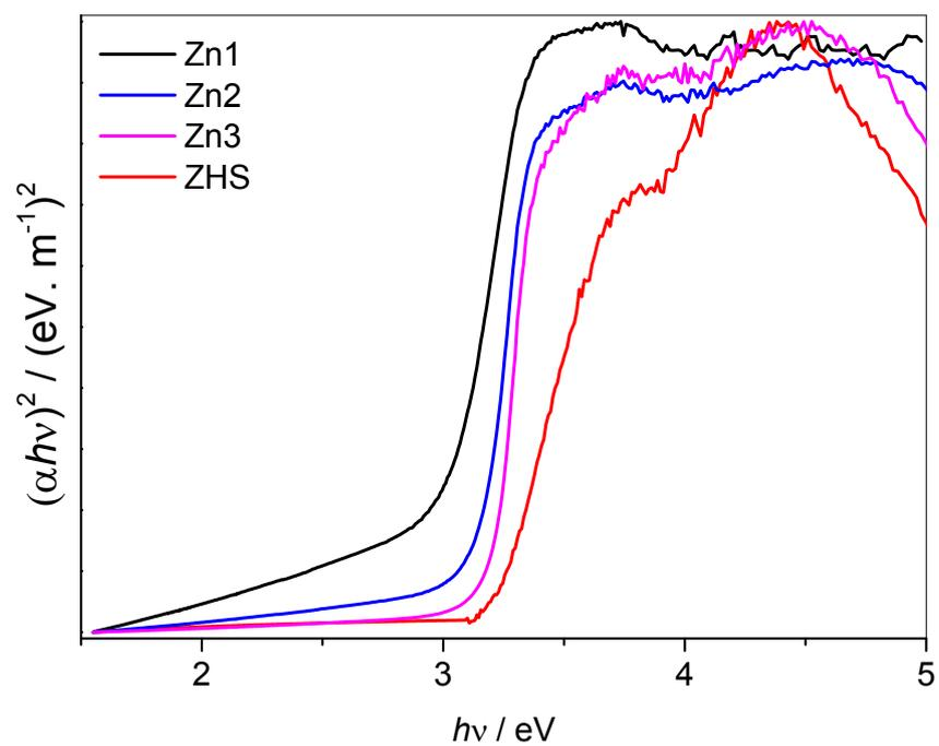
**Figure S12:** Plot of  $(\alpha h\nu)^2$  as a function of  $h\nu$  from the UV-Vis diffuse reflectance curve of as-synthesized samples.
