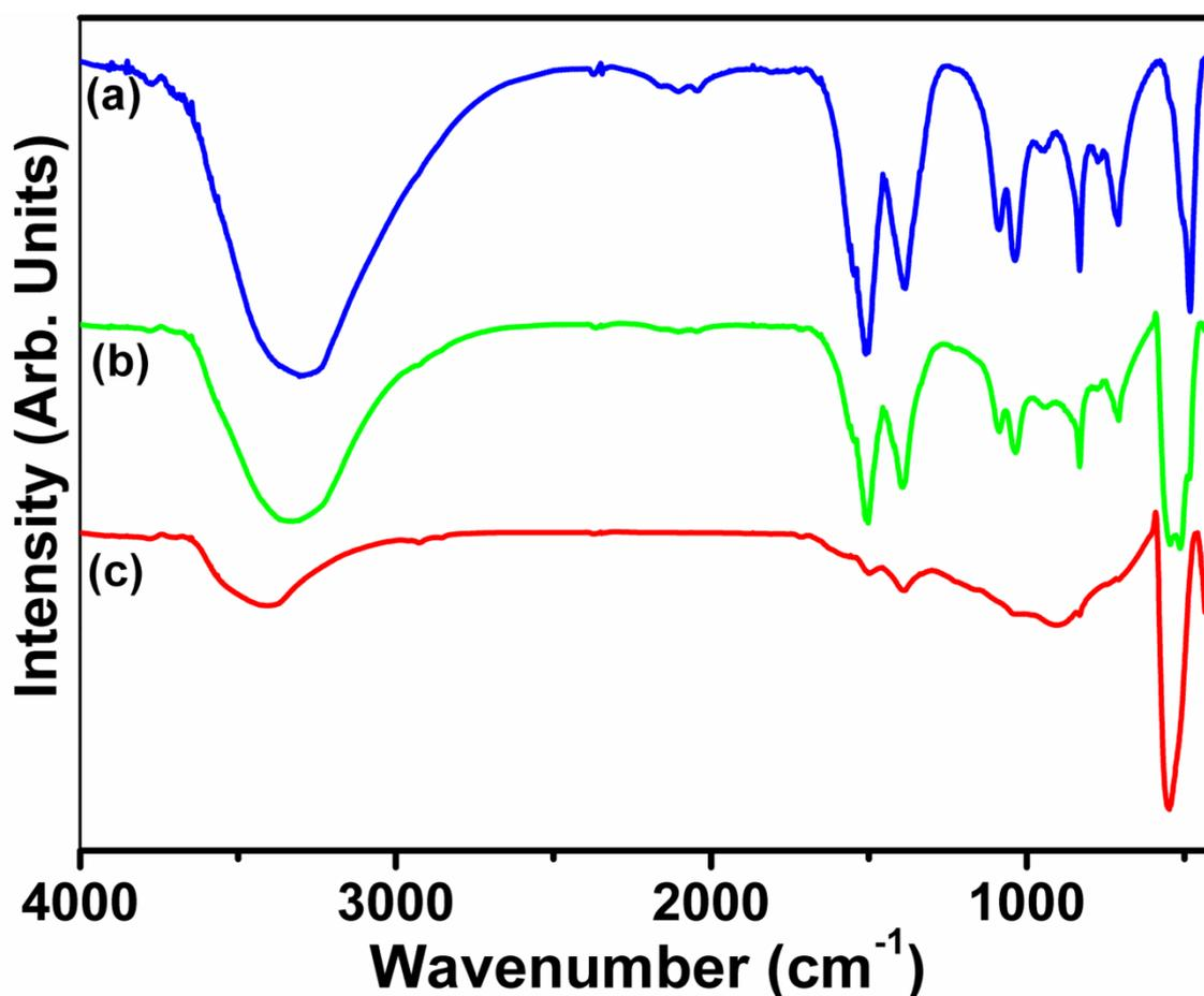
**Figure S11:** Typical FTIR spectra of as-synthesized zinc based hydroxide/oxide samples, (a) Zn-1; (b) Zn-2; and (c) Zn-3.
