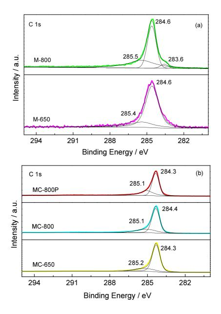
Fig. S1 XPS C 1s spectra of (a) bulk and (b) CNTs supported Mo carbides prepared with DME.
