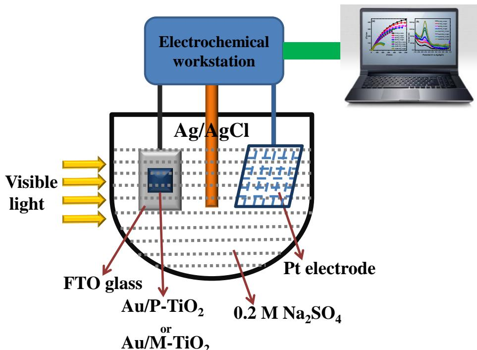
**Fig. S1** Schematic diagram of the photoelectrochemical measurements.
