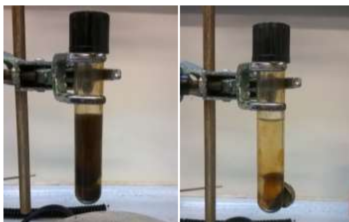
Figure S8. Catalyst recovery using an external magnet of nano-Fe 3 O 4 -dopa@Cp*IrNHC.
