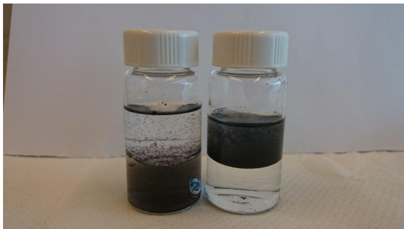
Fig. S3. The original CCS (left) and the CCS after pyrolysis at T = 800\text{ }^{\circ}\text{C} (right) in a biphasic system of water/hexane.
