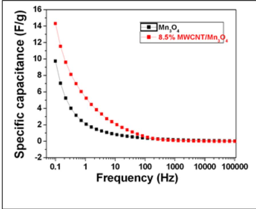
Fig. S1. Frequency dependent specific capacitance of the  $\text{Mn}_3\text{O}_4$  and 8.5% MWCNT/ $\text{Mn}_3\text{O}_4$  composite
