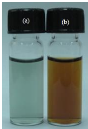
Fig.s2 Optical photographs of the mixture of the CuNCs prepared by the proposed method, 2 mM of free \text{Cu}^{2+} and 20 mM of \text{H}_2\text{O}_2 before (a) and after (b) added 0.5 ml of the \text{Na}_2\text{S} solution (0.1M).
