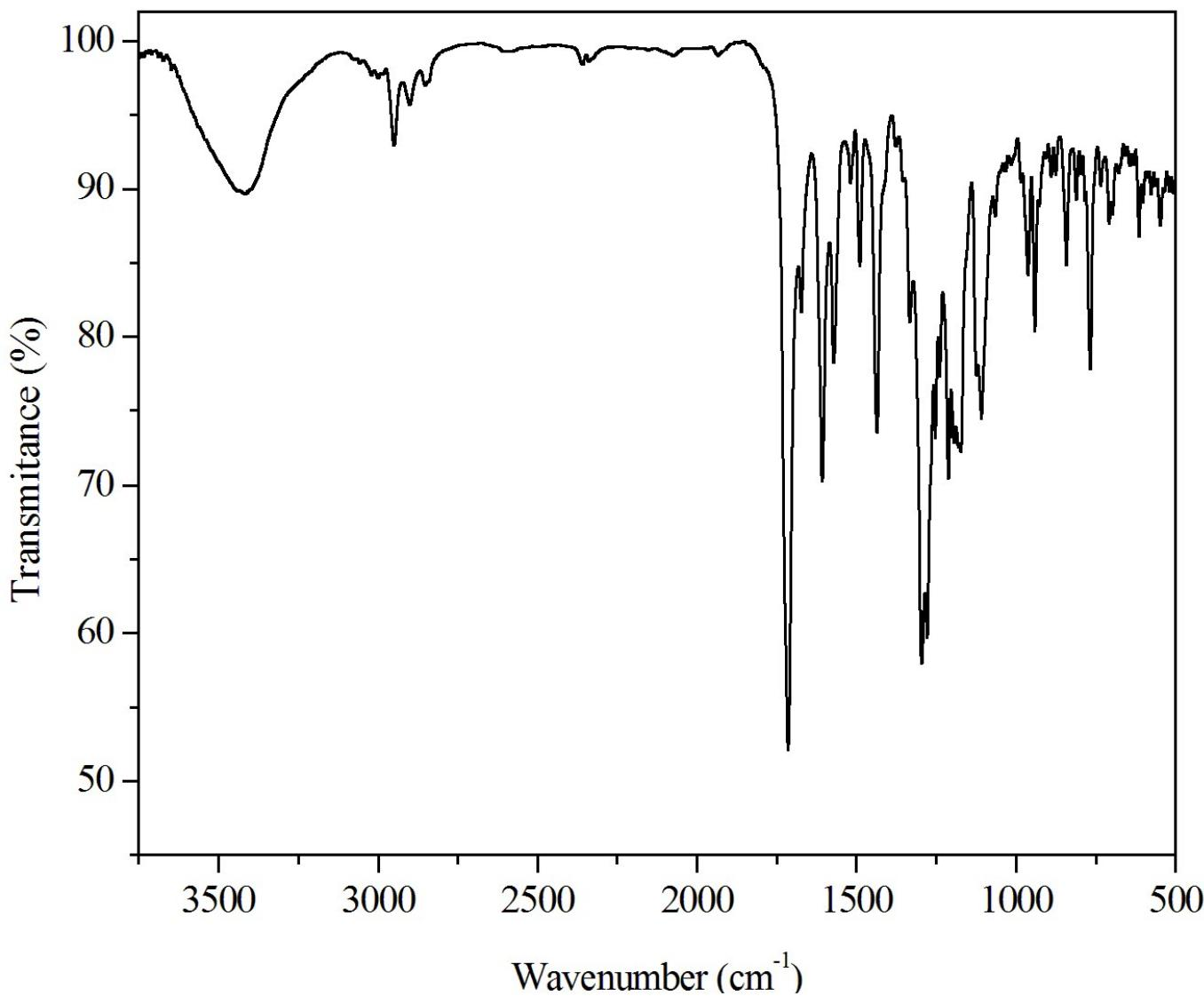
**Fig. ESI8** FTIR spectra of **2c**.
