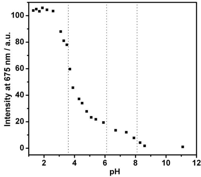
Fluorescence vs pH, for the continuous titration at 675 nm (solid black square), of 2  $\mu\text{M}$   $\text{H}_2\text{TCPPSpm4}$  solution.
