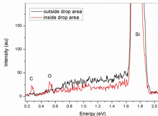
EDS spectra of silicon inside (red line) and outside (black line) the  $\text{H}_2\text{TCPP-Spm4}$  drop spot ( $1\mu\text{M}$ ,  $\text{pH}=8$ ).
