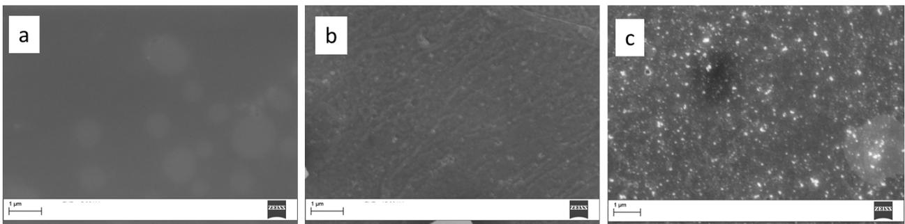
SEM images of  $\text{H}_2\text{TCPPSpm4}$  deposited on silicon by drop casting of  $100\mu\text{l}$  of  $100\mu\text{M}$  solution at  $\text{pH}=1,5$  (a),  $\text{pH}=5$  (b) and  $\text{pH}=8$  (c)
