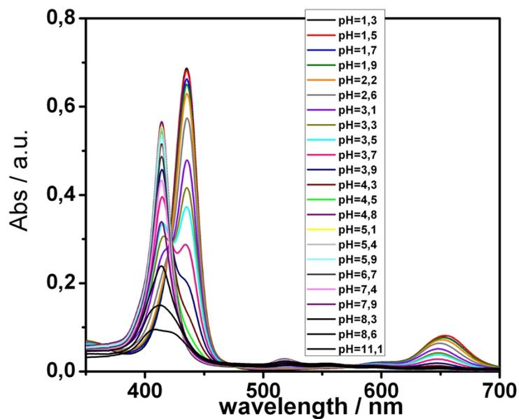
UV-vis spectra of a solution of H<sub>2</sub>TCPPSpm4 (2 μM) increasing the pH from 1.3 to 11.1
