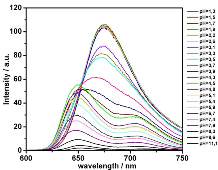
Fluorescence spectra of a solution of H<sub>2</sub>TCPPSpm4 (2 μM) increasing the pH from 1.3 to 11.1. The  $\lambda_{ex}$  424 nm
