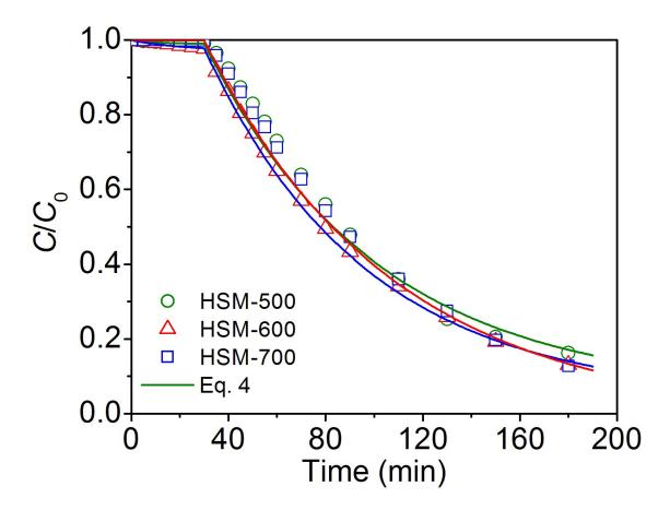
**Fig. S2.** Methylene blue photo-decomposition curves of HSM after calcination at 500, 600 and 700 °C under UV irradiation after adsorption reaction.
