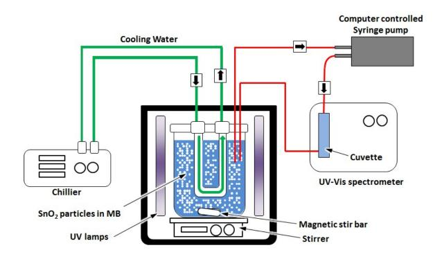
**Fig. S1.** The schematics of the photodegradation apparatus.
