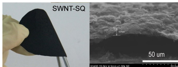
Figure S4 Photographs of flexible nanotubes films and cross-sectional view of SWNT-SQ.
