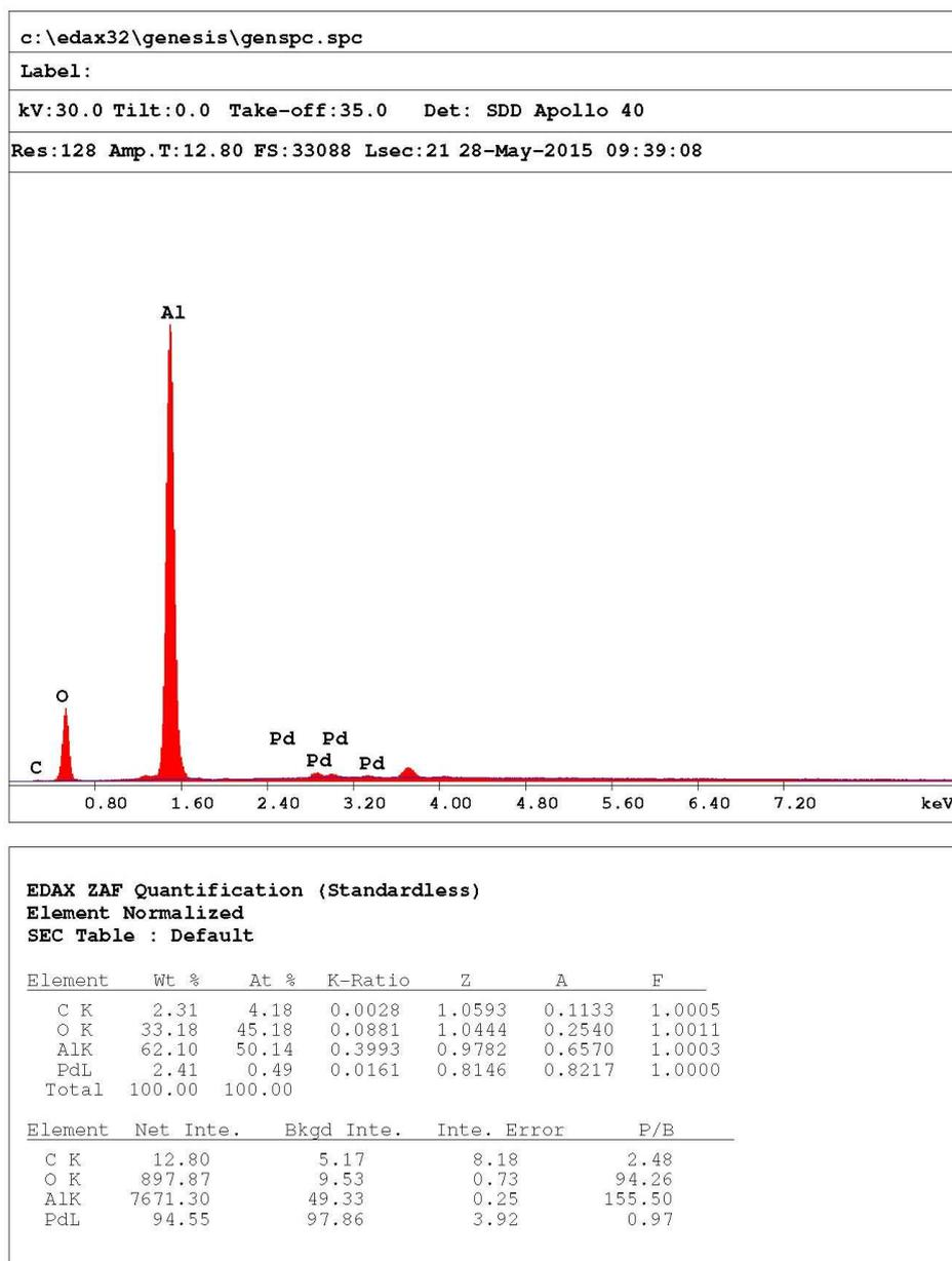
Figure S2 EDX spectrum after using ten times of Pd/AlO(OH) NPs.
