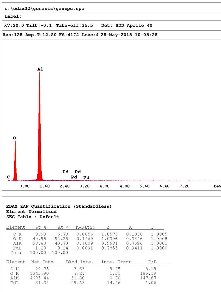
Figure S1 EDX spectrum before the reaction of Pd/AlO(OH) NPs.
