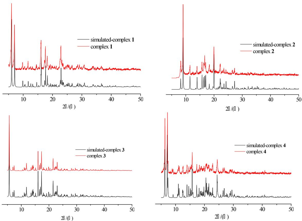
**Figure S2.** X-ray powder diffraction patterns of complex 1-4.
