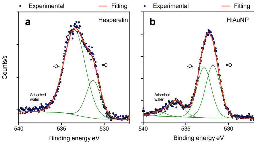
**Figure. S1 XPS measurements** a) Hesperetin O 1s, and d) HtAuNP O 1s envelopes deconvoluted into its components.
