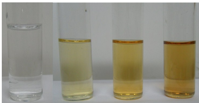
Figure S3. Photographs of various Ag clusters solutions prepared by controlling the pH. The pH (from left to right) was 6.0 (the control), 11.74, 12.08, and 12.75.
