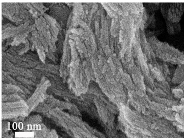
Figure S2. The SEM image of mesoporous Ni-doped  $\text{In}_2\text{O}_3$
