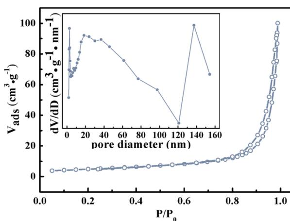
Figure S1. Nitrogen adsorption-desorption isotherms and corresponding pore size distribution(inset) of Ni-doped  $\text{In}_2\text{O}_3$  without SBA-15
