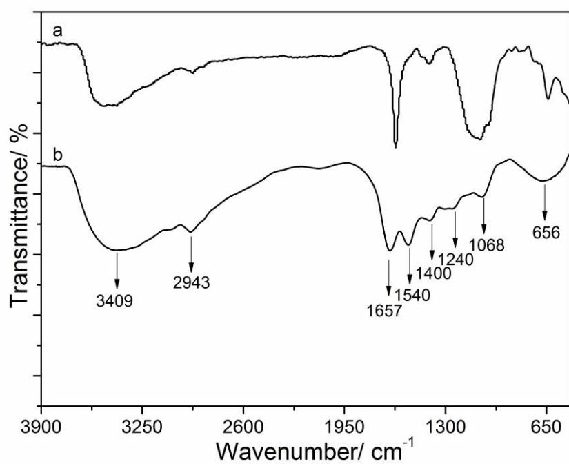
Fig S2. The FT-IR spectra of the uncapped CdS precipitation (curve a) and BSA-CdS QDs (curve b).
