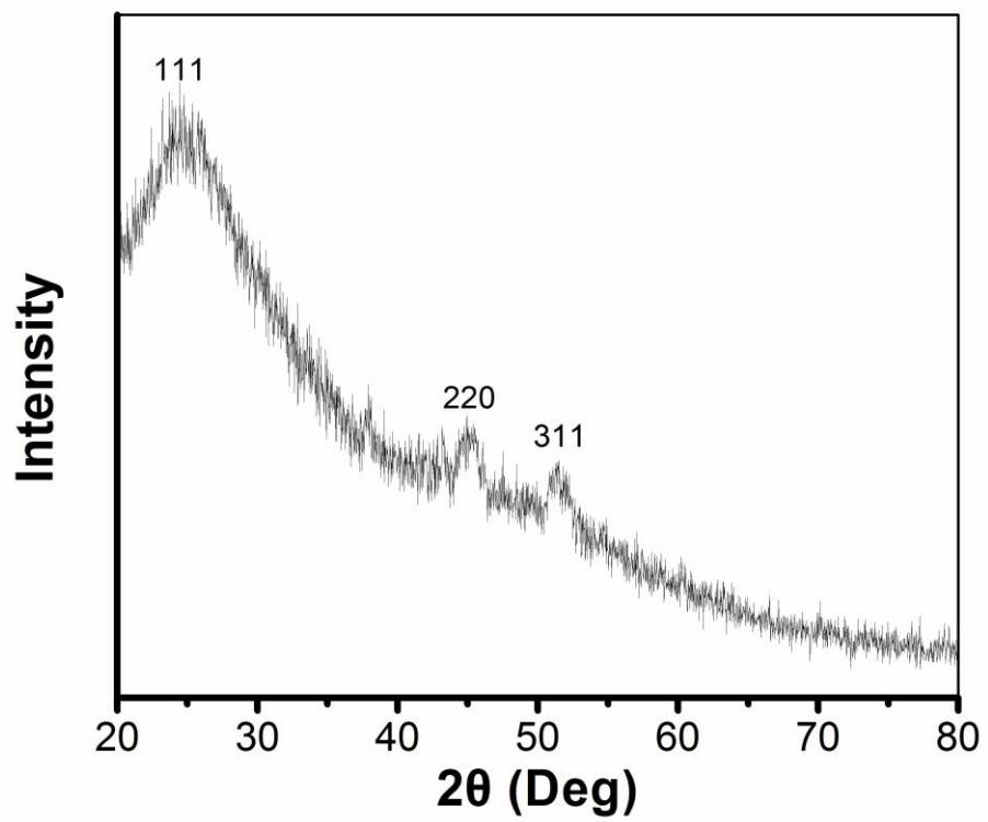
Fig S1. The XRD pattern of BSA-CdS QDs.
