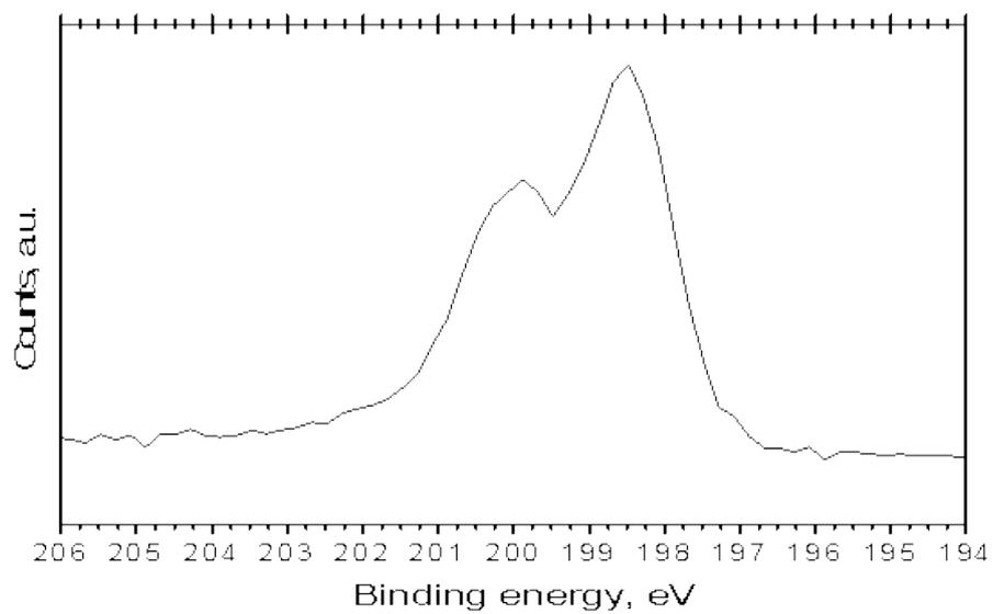
**Figure 3S. Cl<sub>2p</sub> X-ray photoelectron spectroscopy band-like spectrum obtained for MWCNT-CMC-m.**
