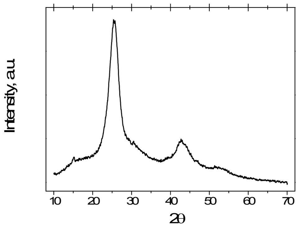
**Figure 2S. X-ray diffraction patterns obtained for pristine multi-walled carbon nanotubes.**
