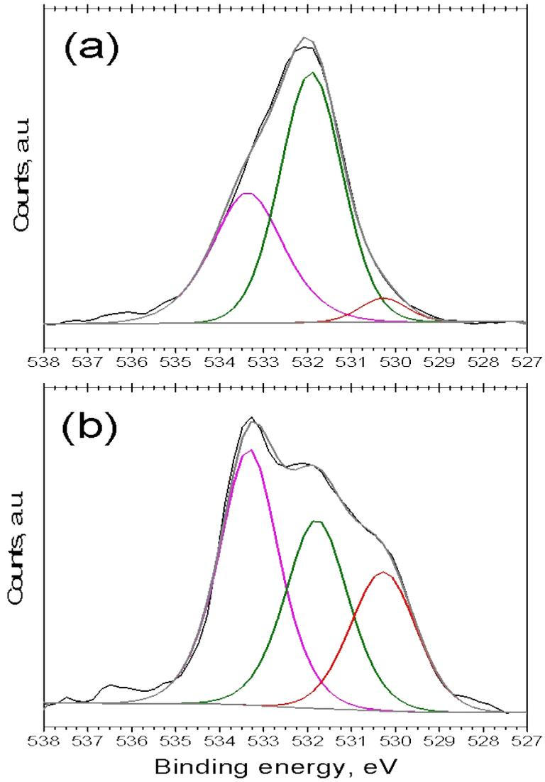
**Figure 4S. O1s X-ray photoelectron spectroscopy band-like spectra (black solid lines) and deconvoluted curves (colored solid lines) obtained for (a) MWCNT-CMC-m and (b) MWCNT-CMC-m-550.**
