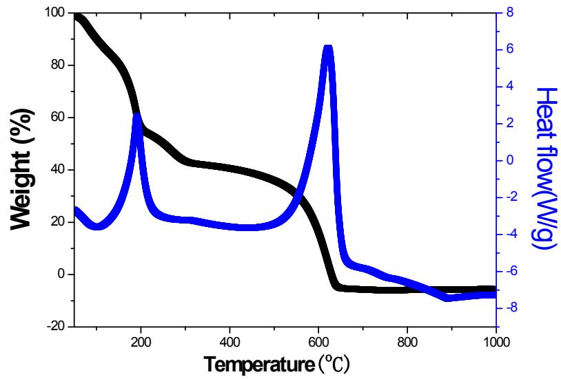
Fig. S1. The thermal analysis curve of graphite oxide
