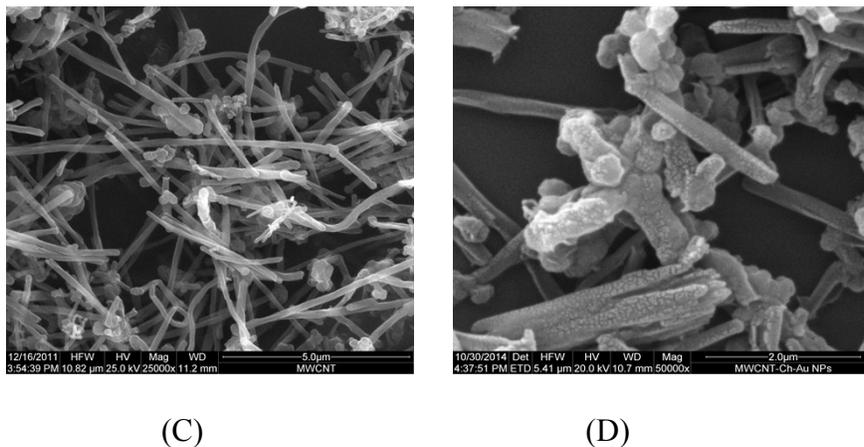
**Figure S4.**(A) SEM-image of graphene (GR) sheets, (B) for graphene-Ch-Au NPs, (C) for MWCNTs and (D) for MWCNTs-Ch-Au NPs nanocomposites
