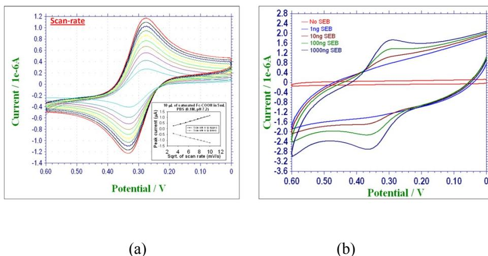
**Figure S13.** (a) Cyclic voltammograms at different scan rates for ferrocene carboxylic acid and (b) is the cyclic voltammograms at different concentrations of SEB at [GR-Ch-Au NPs-CAB-SEB-Fc-MAB] modified electrode at 50mV/s scan rate.
