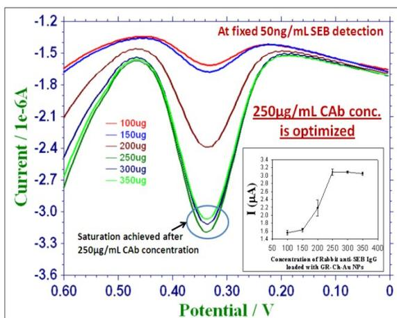
**Figure S10.** SWV obtained for immunosensing of 50ng/mL SEB at different concentrations (100, 150, 200, 250, 300 and 350 $\mu$ g/mL) of rabbit anti-SEB polyclonal IgG [CAb] in their [GR-Ch-Au NPs-CAb] bionanoconjugates
