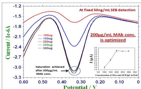
**Figure S8.** SWV obtained for immunosensing of 50ng/mL SEB at different concentrations (100, 150, 200, 250 and 300 $\mu$ g/mL) of mice anti-SEB monoclonal IgG [MAb] in their [Fc-MAb] bioconjugates
