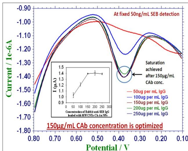
**Figure S12.** SWV obtained for immunosensing of 50ng/mL SEB at different concentrations (50, 100, 150, 200 and 250µg/mL) of rabbit anti-SEB polyclonal IgG [CAb] in their [MWCNTs-Ch-Au NPs-CAb] bionanoconjugates
