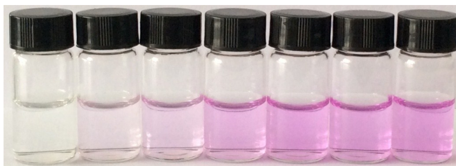
Fig. S6 Color changes of PEGRh in aqueous solution (10 \mu\text{M} ) upon addition of varying quantities of \text{Cu}^{2+} ions (from left to right: 0, 0.05, 0.1, 0.25, 0.5, 1.0, 2.0 equiv.).
