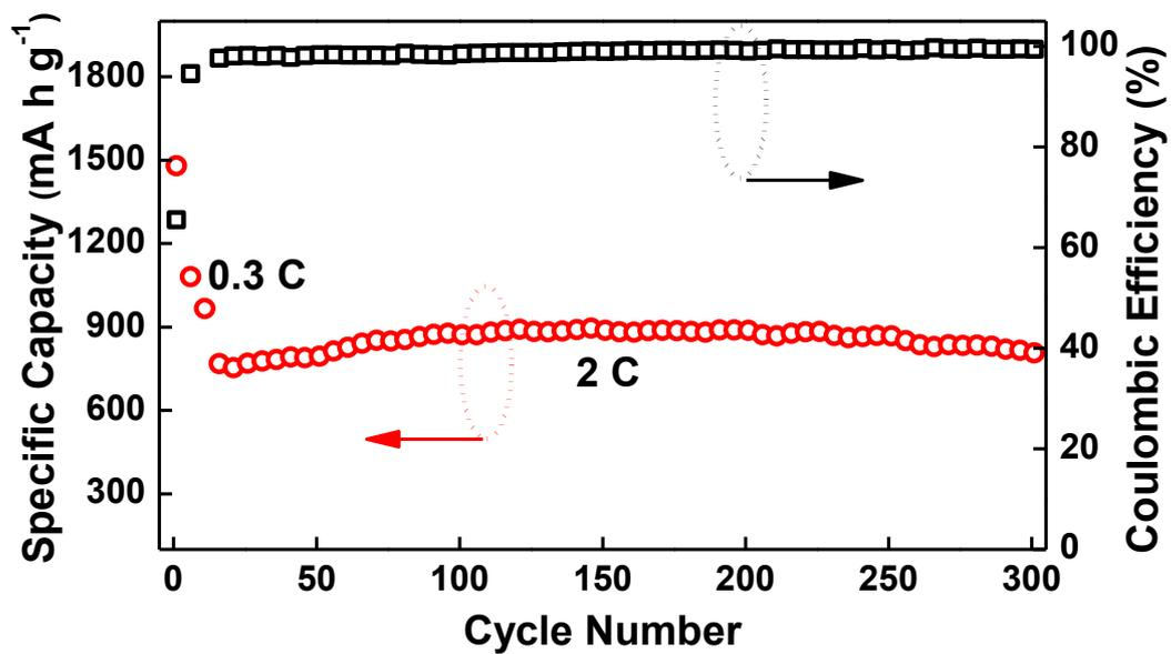
**Figure S6.** Cycling performance of the Fe<sub>3</sub>O<sub>4</sub>/C microrods electrode at a current density of 2 C (1 C=1000 mA g<sup>-1</sup>). The electrode was firstly activated at 0.3 C for the initial 10 cycles.
