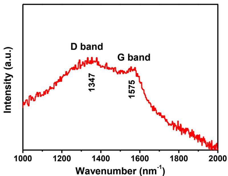
**Figure S3.** Raman spectrum of the as-prepared Fe<sub>3</sub>O<sub>4</sub>/C microrods. The high intensity of D band relative to G band indicates the amorphous nature of the carbon material.
