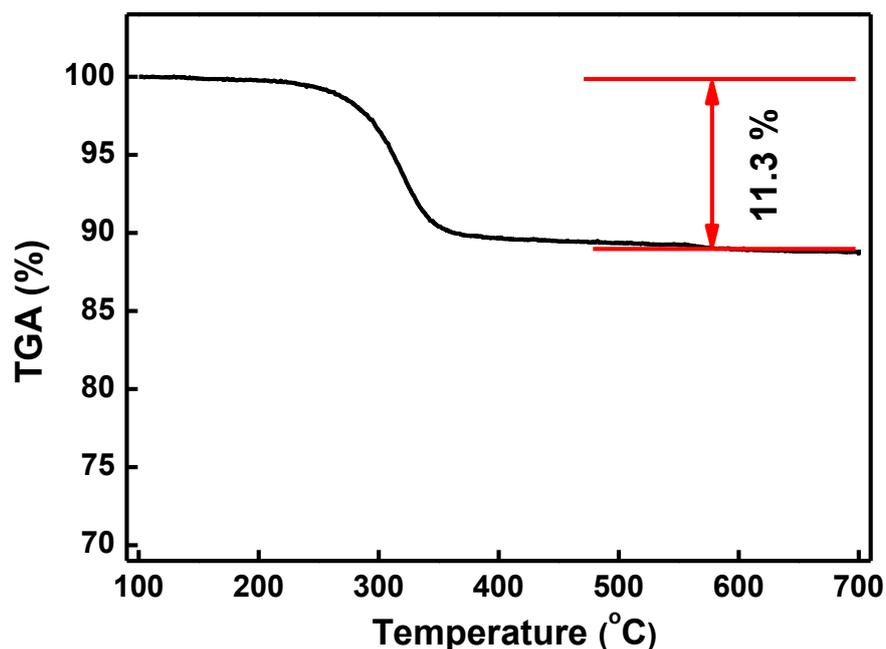
**Figure S4.** TGA curve of the as-prepared  $\text{Fe}_3\text{O}_4/\text{C}$  microrods from 100 to 700 °C under air gas flow with a temperature ramp of 10 °C  $\text{min}^{-1}$ .
