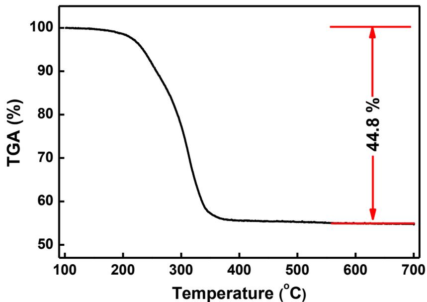
**Figure S2.** TGA curve of the as-prepared Fe-glycolate precursor from 100 to 700 °C under N<sub>2</sub> gas flow with a temperature ramp of 10 °C min<sup>-1</sup>.
