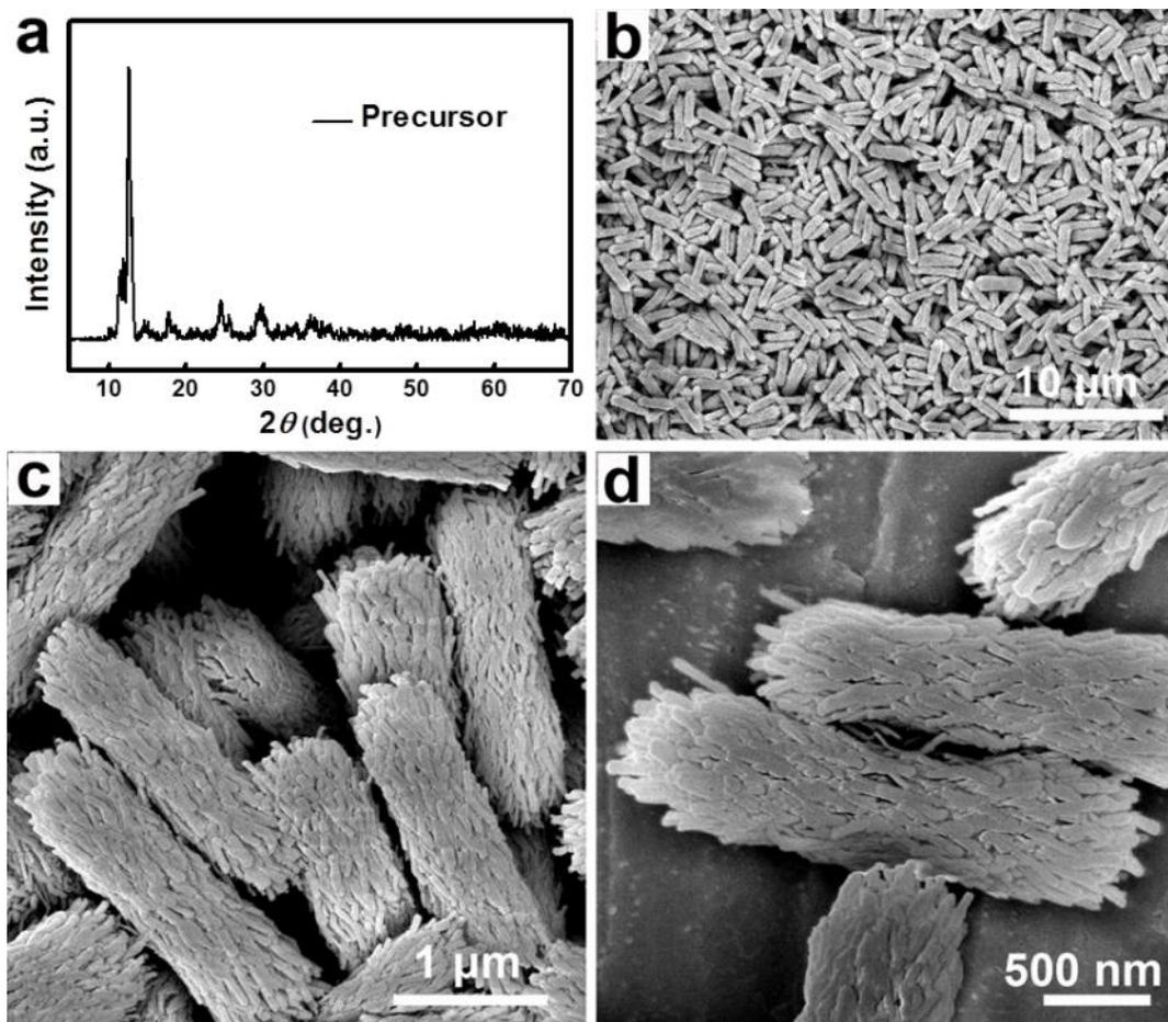
**Figure S1.** (a) XRD pattern and (b-d) FESEM images of the as-prepared Fe-glycolate precursor microrods.
