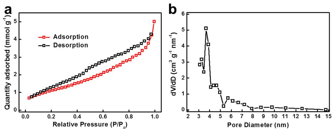
**Figure S5.** (a)  $\text{N}_2$  adsorption-desorption isotherm plots and (b) corresponding BJH pore size distribution of the  $\text{Fe}_3\text{O}_4/\text{C}$  microrods.
