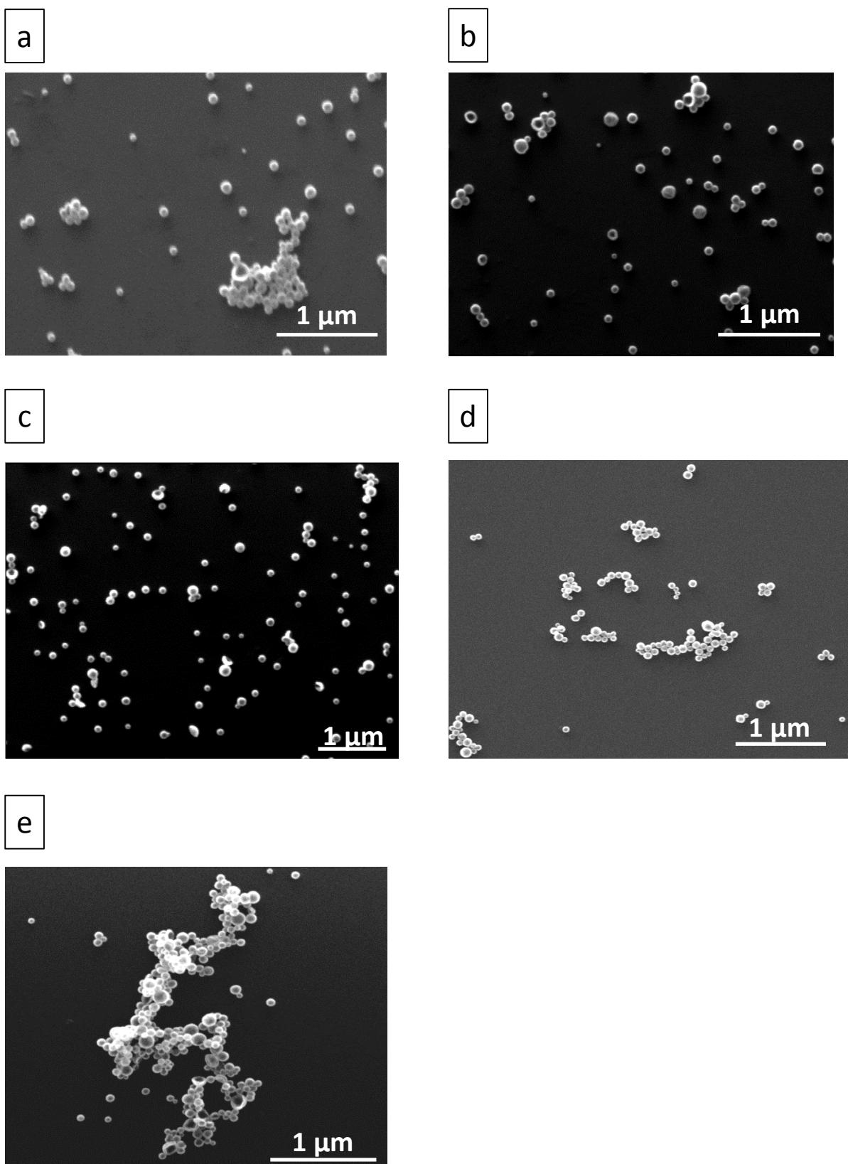
**Figure S 1:** SEM images corresponding to extinction spectra in Figure 1, (a) PVP-stabilised HGNs, (b) PAM-stabilised HGNs, (c) thioglucose-stabilised HGNs, (d) silica-stabilised HGNs, and (e) dextran-stabilised HGNs.
