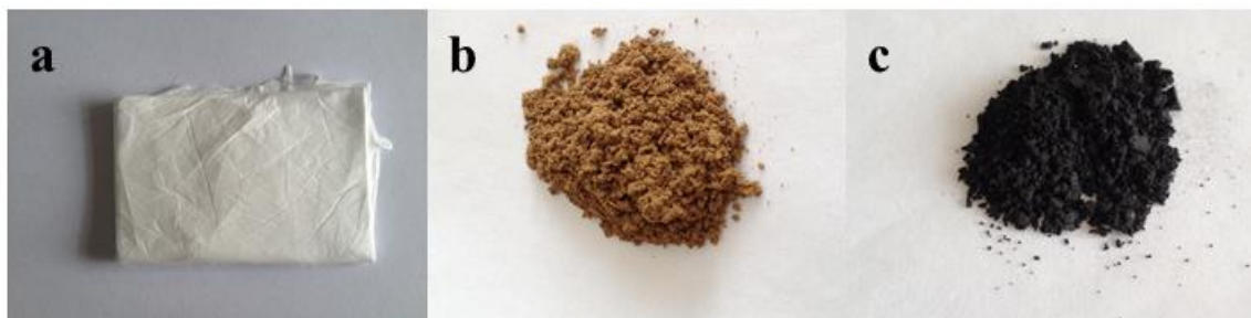
Figure S1. Digital images of the (a)SiO 2 nanofibres; (b)pure Si nanofibres synthesized by directly magnesiothermic reduction; (c) Si NP@C nanofibres.
