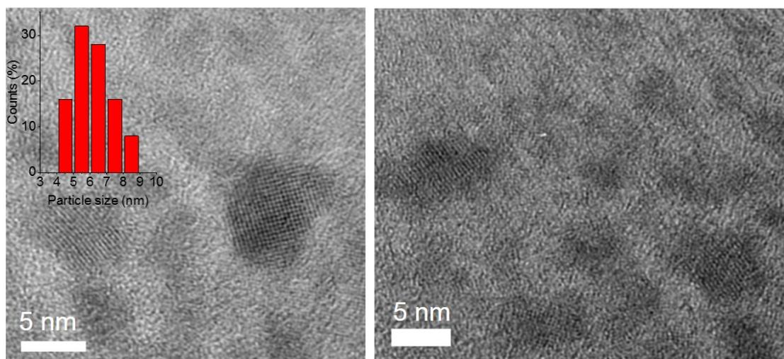
**Fig. S4** Typical TEM images of 3-APA-capped BiFeO<sub>3</sub> NPs. Inset: the corresponding particle size distribution, indicating an average particle size of 6.2 nm. The particle size distribution was estimated by measuring the size of about 100 individual nanoparticles in several TEM images.
