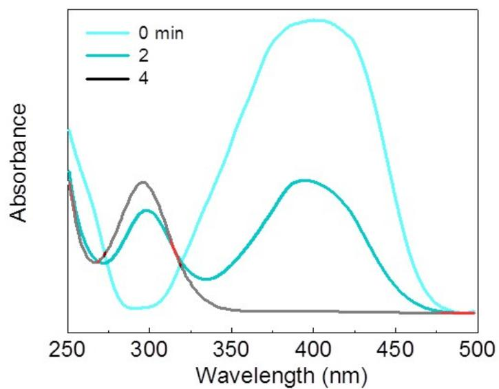
**Fig. S7** Time-dependent UV-vis absorption spectra for *p*-nitrophenol reduction by  $\text{NaBH}_4$  in the presence of MBFAs catalyst.
