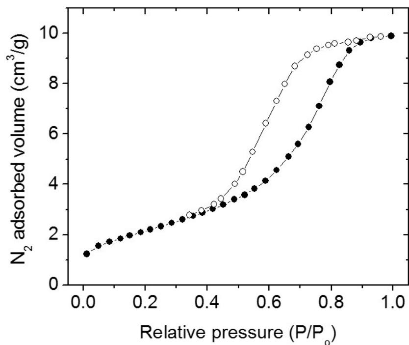
**Fig. S6** Nitrogen adsorption–desorption isotherms at 77 K of randomly aggregated BiFeO<sub>3</sub> NPs, showing BET surface area of ~8 m<sup>2</sup>g<sup>-1</sup> and total pore volume of ~0.01 cm<sup>3</sup>g<sup>-1</sup>.
