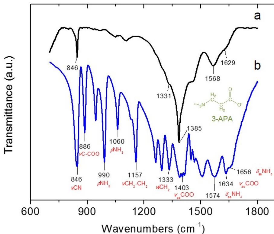
**Fig. S1** Infrared spectra for (a) BiFeO<sub>3</sub> NPs capped with 3-aminopropanoic acid (3-APA) ligands and (b) pure 3-aminopropanoic acid compound. The assignment of IR peaks of 3-APA to various vibration modes was based on that of ref. [18] ( $\nu$  - stretching,  $\delta$  - bending,  $w$  - wagging,  $\rho$  - rocking,  $s$  - symmetric,  $as$  - asymmetric).
