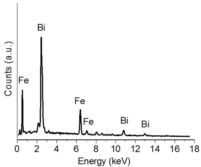
**Fig. S5** Typical energy-dispersive X-ray spectroscopy (EDS) spectrum of MBFAs, showing a Bi:Fe atomic ratio of ~1:1.
