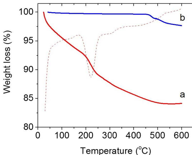
**Fig. S3** TG profiles (solid lines) performed in air of (a) as-prepared containing surfactant and (b) mesoporous MBFAs sample. The differential thermogravimetric (DTG) curve (dashed lines) for as-prepared materials is also given.
