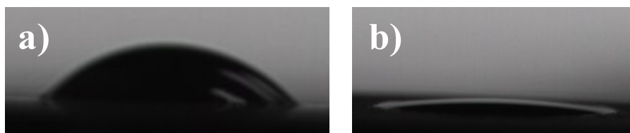
Figure S3. Shapes of a PDMS prepolymer on the hierarchical (a) Ni surface and (b) Ni/NiO surface (obtained after heating at 500 °C). The PDMS prepolymer has a lower contact angle on the Ni/NiO surface, which can facilitate the entering of the prepolymer into the templates.
