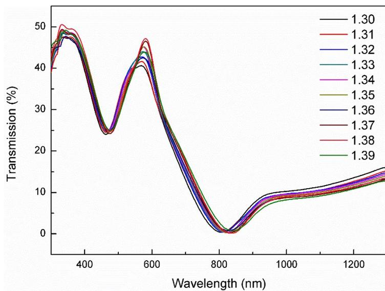
**Fig. S5** Experimentally determined transmissions of the PNPA for liquids with refractive indices of 1.30– 1.39 in steps of 0.01 RIU.
