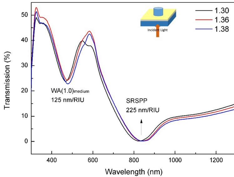
**Fig. S6** Experimentally determined transmission spectra of the PNPA without nanodisks for liquids with refractive indices of 1.3, 1.36, and 1.39. In the case of the structure composed of a resist nanopillar array and a perforated metal film, the sensitivity of WA(1.0)<sub>medium</sub> and SRSPP was only 125 and 225 nm/RIU, respectively. The sample was realized by removing the top metal layer with adhesive tape.
