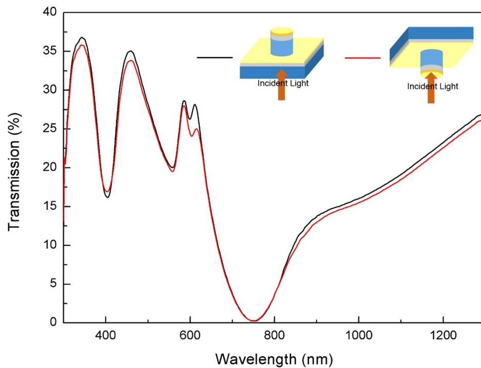
**Fig. S4** Experimentally determined transmissions of the PNPA with the light incident from both sides. No noticeable difference was observed in the transmissions.
