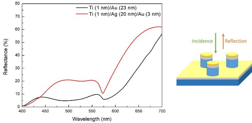
**Fig. S3** Simulated reflectance spectra of PNPA structures with Ti (1 nm)/Au (23 nm) and Ti (1 nm)/Ag (20 nm)/Au (3 nm) layers. The PNPA with the Ag layer exhibited a higher reflectance and a distinct spectrum within the visible range; this resulted in better visual perception.
