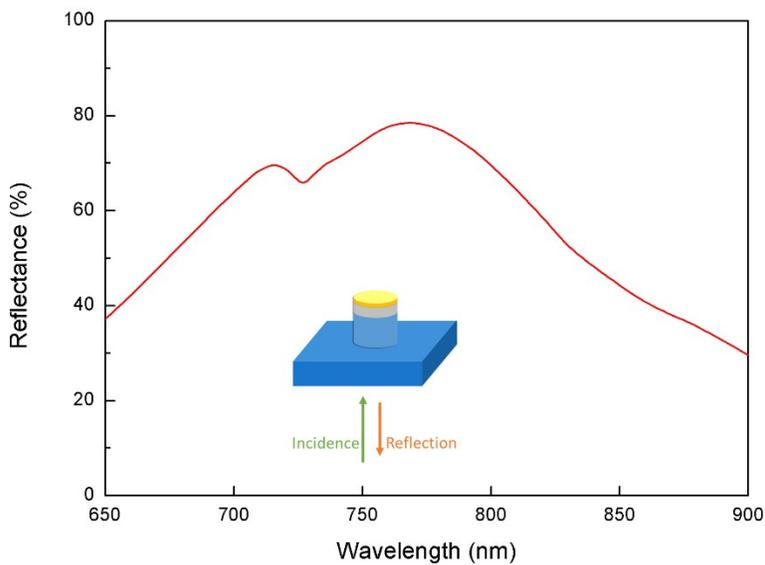
**Fig. S2** Simulated reflectance spectrum of the metal nanodisk array supported by the nanopillars. The structure shows a high reflection for wavelengths of 750– 850 nm.
