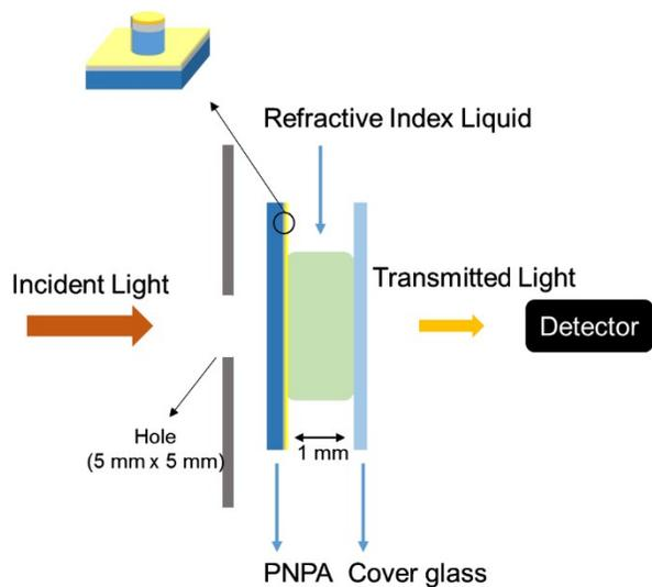
**Fig. S1** Experimental setup for measuring the transmission spectrum of the PNPA for various refractive index liquids. The experiments were performed with a SolidSpec-3700DUV spectrophotometer (SHIMADZU).
