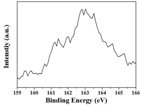
**Figure S2** S 2p XPS spectra of the as-spun  $\text{Li}_2\text{S}_3\text{-C}$  NFs
