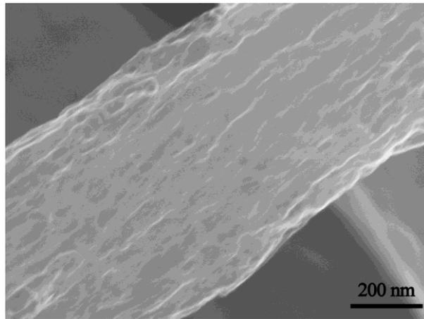
Figure S4 SEM image of a Carbon fiber with the absence of  $\text{Li}_2\text{S}$ .
