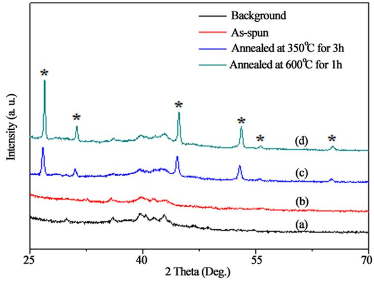
Figure S1 XRD patterns for as-spun and annealed samples, respectively.
