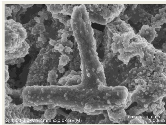
Figure S5 The SEM image of  $\text{Li}_2\text{S}$ -C NFs after CV scan for 5cycles
