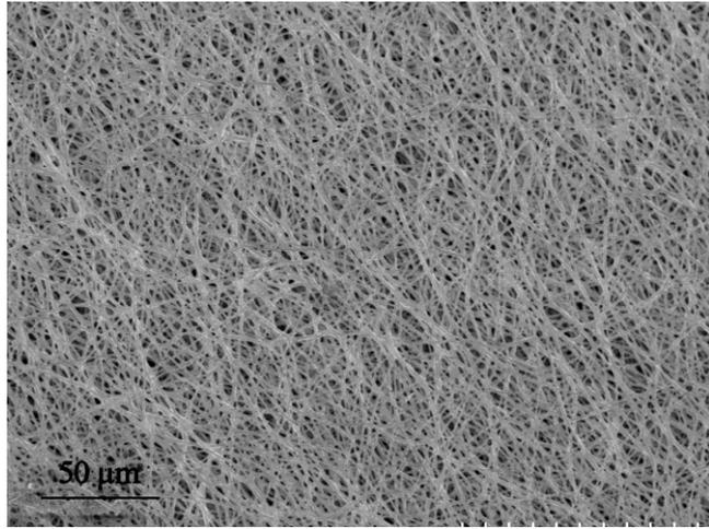
Figure S3 SEM image of as-spun  $\text{Li}_2\text{S}_3$ -PVP composites.
