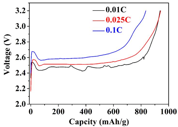
Figure S6 Initial charge curves at a rate of 0.01C, 0.025C and 0.1C, respectively.
